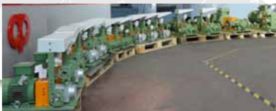
Metering pumps "N" for Borouge 3 plant.
